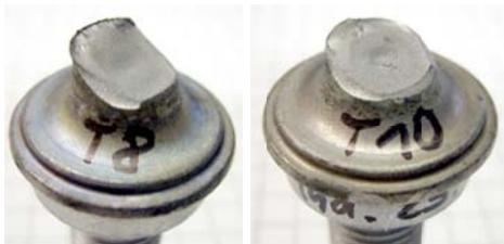
Figure 2: Fracture patterns of welded ball stud
