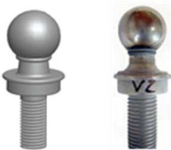
Figure 1: Ball stud as a model and in original, welded design
