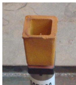
Figure 1. Standard thermoanalysis croning sand cup with K type thermocouple
